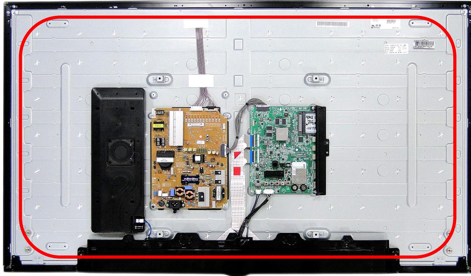
After turning on the power and disassembling the case, check with the naked eye, whether you can see light from module holes.
