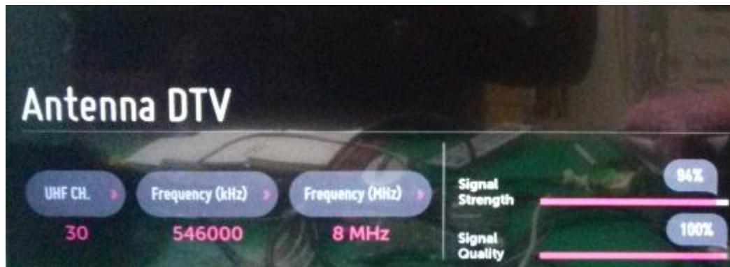
When the signal is strong, use the attenuator (-10dB, -15dB, -20dB etc.)
